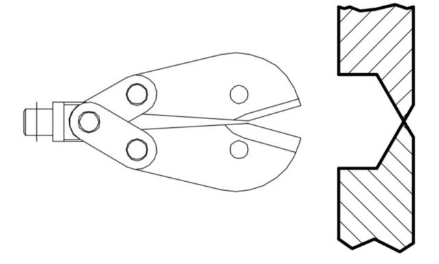
Spare head for MRC8 - pneumatic cutter - side cutter
